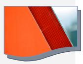
visibility as the marking material appears brighter. The outer red part of this SMV emblem is retroreflective while the inner orange part is a nonreflective material
